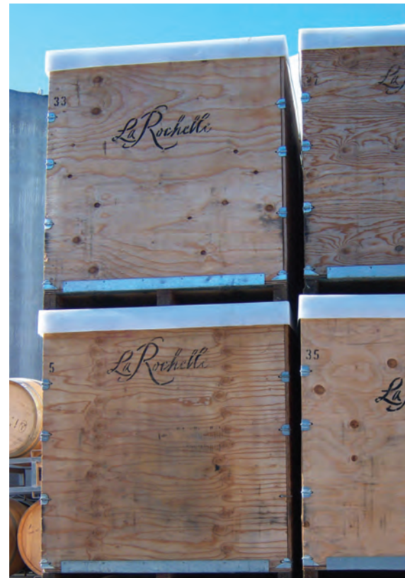
Steven Kent and La Rochelle use wood boxes with plastic liners for primary fermentation. The boxes hold 1.5 to 1.7 tons and can be moved and stacked with forklifts.
